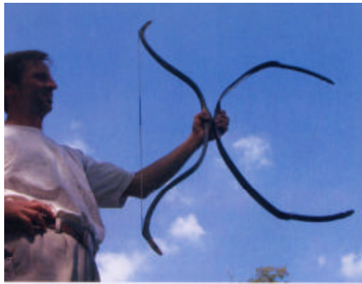
Bowyer Lukas Novotny demonstrates the C-shape of the unstrung recurved bow, which, when strung, takes on its characteristically serpentine, tips-forward shape.
