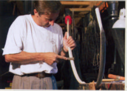
1. Water-buffalo horns await shaving, cutting, steaming and gluing to a wooden core in Novotny's Ohio workshop. 2. Building blocks of a Turkish-style composite bow: two strips of horn, two dustar limbs, two siyahs (attached), a grip and two bundles of sinew; the finished bow at the top shows the final unstrung shape. 3. After gluing horn to the inside of the core, Novotny lays down sinew on the outside of the dustar . 4. He combs the sinew, which will then dry for weeks, pulling the tips of the bow ever closer together. When the bow is curved back, the sinew will be stretched, giving the bow far more power than if it were made only of wood. 5. After a year of seasoning, Novotny uses molded forms called tepeliks to pull the bow into stringing position.
